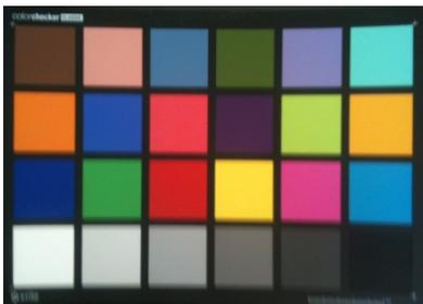
**Figure S9.2.** X-Rite ColorChecker Classic card used to verify camera color balance and sensitivity prior to and during field deployment. The card is available online for about \$70 at B&H Photo, see [www.bhphotovideo.com/c/product/465286-REG](http://www.bhphotovideo.com/c/product/465286-REG).
