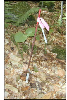
Figure 8 Site marker- forestry tape and rebar
